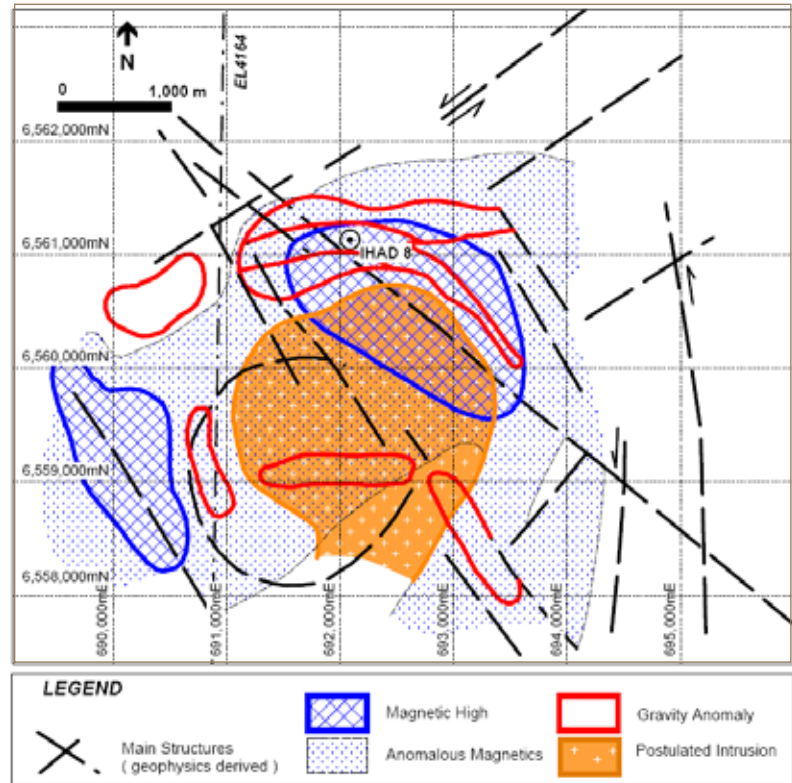
Figure 7: Interpretation plan of key geological elements, Winjabbie East Prospect area, EL4164. Winjabbie East occurs at the intersection of geophysically defined north-west- and north-east-trending crustal-scale structural corridor.
